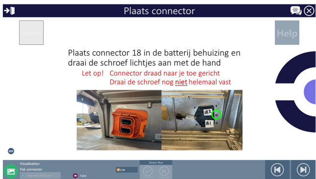
Figure 4. Example of digital work instructions. Translation: insert connector 18 into the battery housing and tighten the screw slightly by hand. Note: keep the connector wire facing you and do not tighten the screw all the way. Source: Authors' own work
