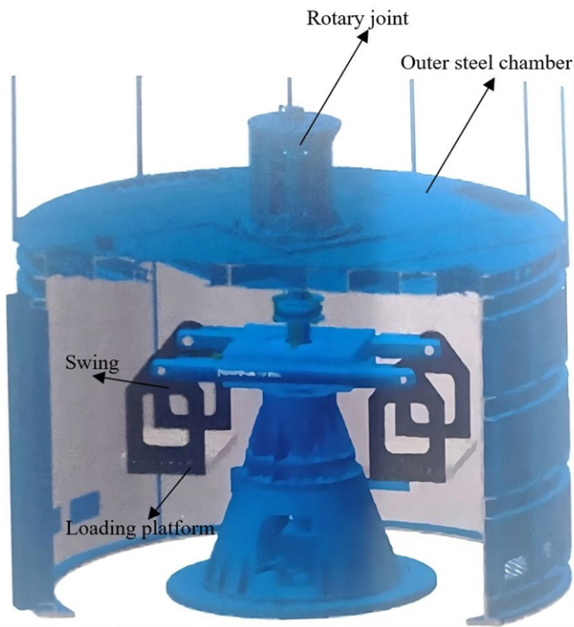
Figure 1. Newly developed TCU Mark III geotechnical centrifuge facility
