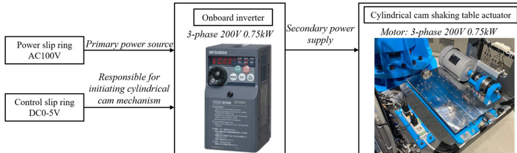
Figure 7. System configuration for the cylindrical cam shake table
