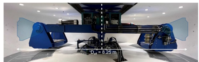
Figure 1. The 500 gtonne capacity ETHZ beam centrifuge
