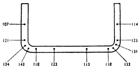
FIG. 35.—EFFECT OF COLD-FORMING ON A SIMPLE CHANNEL
