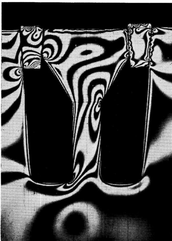
FIG. 22: PHOTOELASTIC FRINGE PATTERN FOR THE ASYMMETRIC CASE
