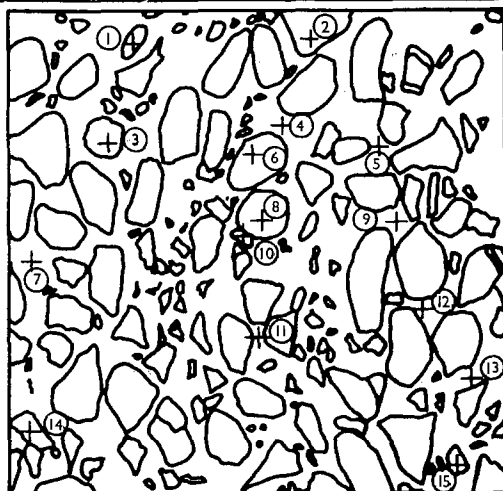
Crushed gravel max. agg. size 19 mm
