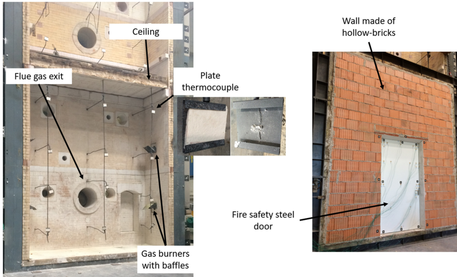
Figure 1. Fire resistance test furnace (left) and wall made of bricks with embedded steel door (right)
