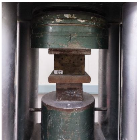
Figure 6. Compressive strength test showing the heated sample under the ConTest compression machine. Authors' own work
