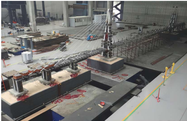
Figure 8. Test model of an ultra-large span cable-stayed bridge
