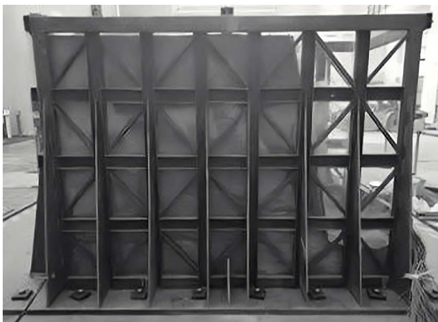
Figure 9. Mold box after casting
