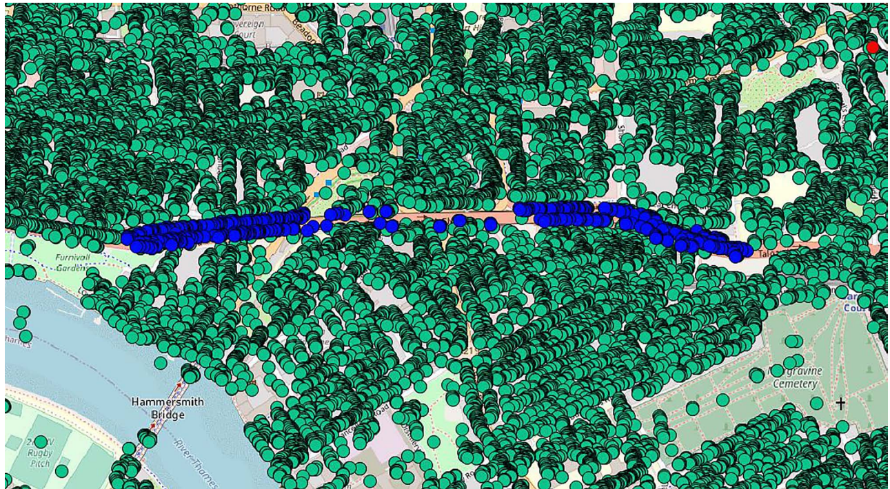
Figure 9. Outcome of the selection process to identify persistent scatterers associated with the bridge (marked in blue) from other persistent scatterers (marked in green). The GCP used in the InSAR processing of the Sentinel data and 2015–2018 Cosmo-SkyMed data is marked in red
