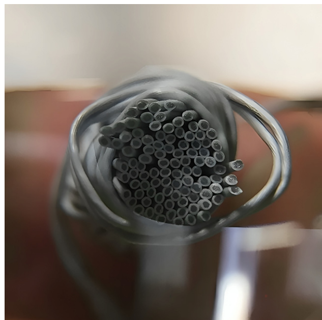
Figure 17. Magnified section through polyester yarns with PVC coating
