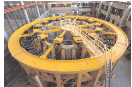
Figure 2. The full-scale tunnel test facility at the Delft University of Technology in the Netherlands. The facilities diameter and height are 16 m and 6 m
