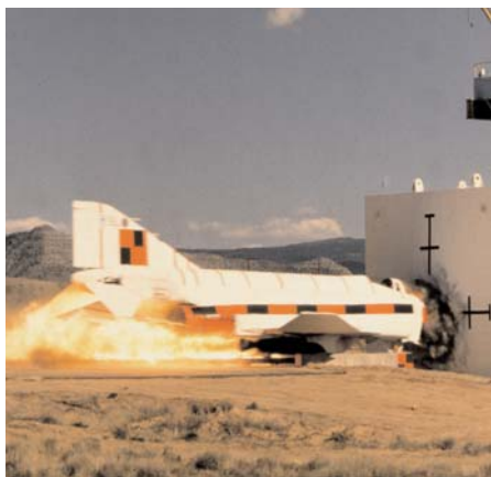
Experimental research in cooperation with Japan and the US: simulation of airplane impact on concrete protection wall
