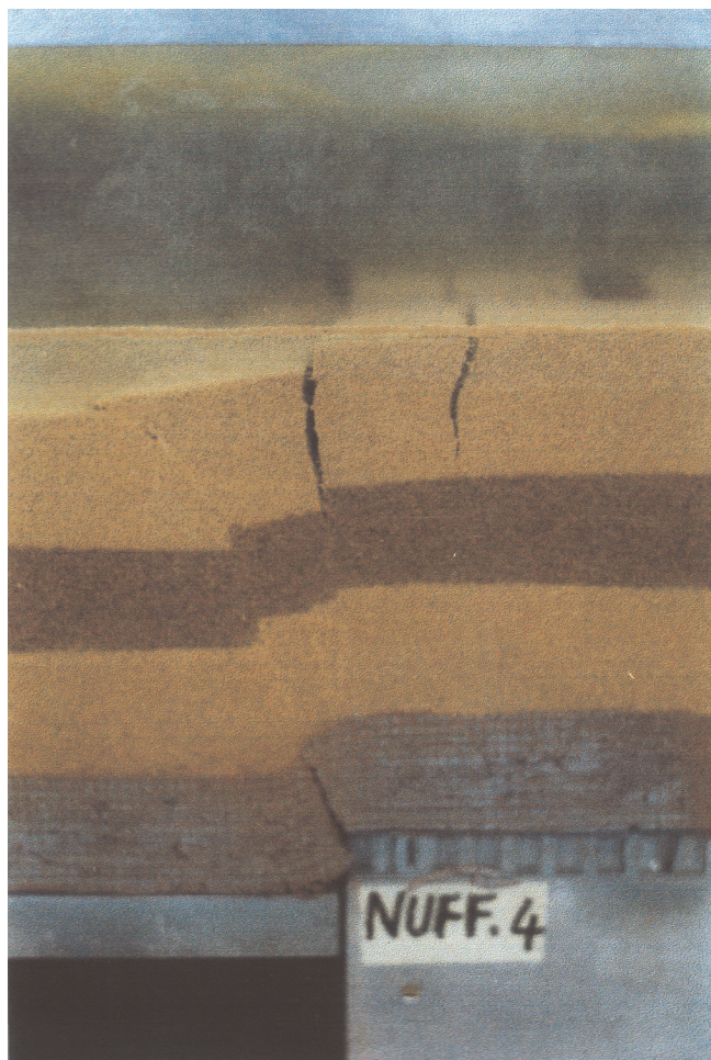
Figure 10. Clay barrier, 500 mm displacement
