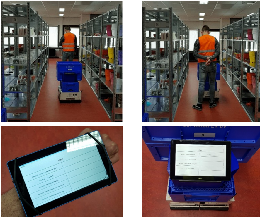
Figure 4. HRC settings. Left: Human leading and robot following. Right: Human following and robot leading
