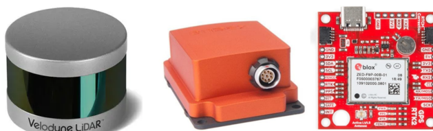
Figure 4. Velodyne VLP-16 LIDAR sensor (left), XSense MTI-100 IMU (centre), Sparkfun GPS-RTK2 Board – ZED F9P (right). https://www.aeroexpo.online/de/prod/velodyne/product-176220-32079.html , https://www.mouser.de/ProductDetail/Movella-Xsens/MTI-100-2A8G4?q_s=B6kkDfuK7%2FD4DcRKGaHtg%3D%3D , https://www.sparkfun.com/sparkfun-gps-rtk2-board-zed-f9p-qwiic-gps-15136.html . Source: Authors' own work
