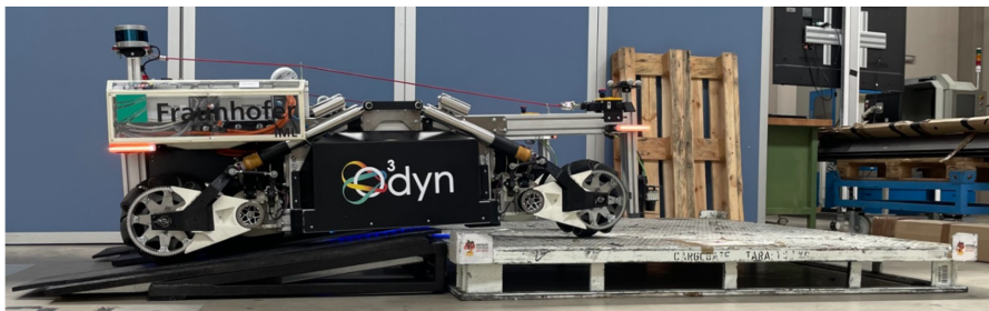
Figure 9. O 3 dyn transitioning onto an LSP via the ramp in the laboratory. Source: Authors' own work
