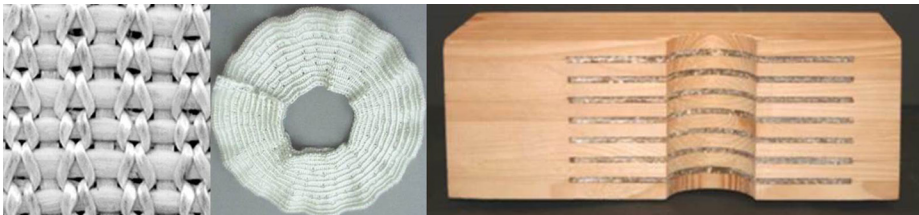
Plate 4. Surface view of plain Jersey with warp and weft insertion; spiral disc of biaxial knitted reinforcement; and placement of reinforcement in wooden test specimen (Haller et al. , 2006)
