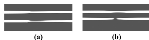
Figure 19 Illustration of experimental (top) width and simulation (bottom) of flow rate from results for 0.3 mm layer height and (a) acceleration region for K_{LA} = 0 and (b) deceleration region for K_{LA} = 0.0 . Edges traced using the software Inkscape for image clarity
