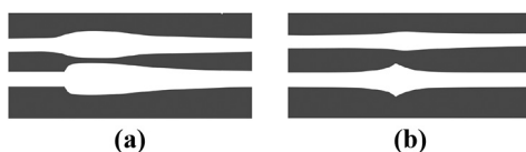
Figure 18 Illustration of experimental width (top) and simulation of flow rate (bottom) results for 0.3 mm layer height and (a) acceleration region for K_{LA} = 0.2 and (b) deceleration region for K_{LA} = 0 . Edges traced using the software Inkscape for image clarity
