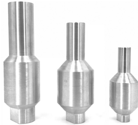
Figure 3 Manufactured aluminum go/no-go gauges for verification
