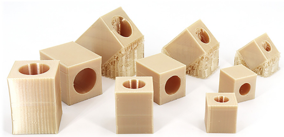
Figure 1 Specimens with FDM-printed holes
