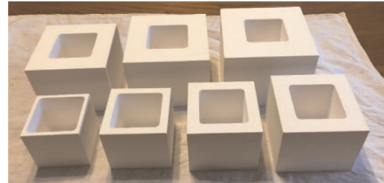
Figure 2 Open molds used for the SP.2
