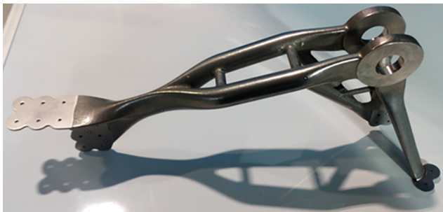
Figure 15 Component manufactured by Arcam, post-processed by centrifugal finishing and milled to achieve specific tolerances
