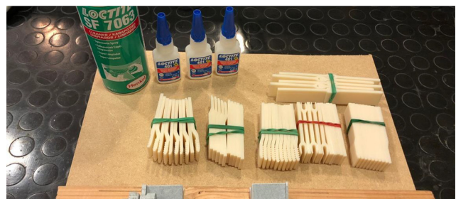
Figure 4 3D printed specimens before bonding with Loctite 401
