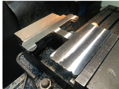
Figure 14 "Part 1" built with enhanced-pixel strategy after top surface machining
