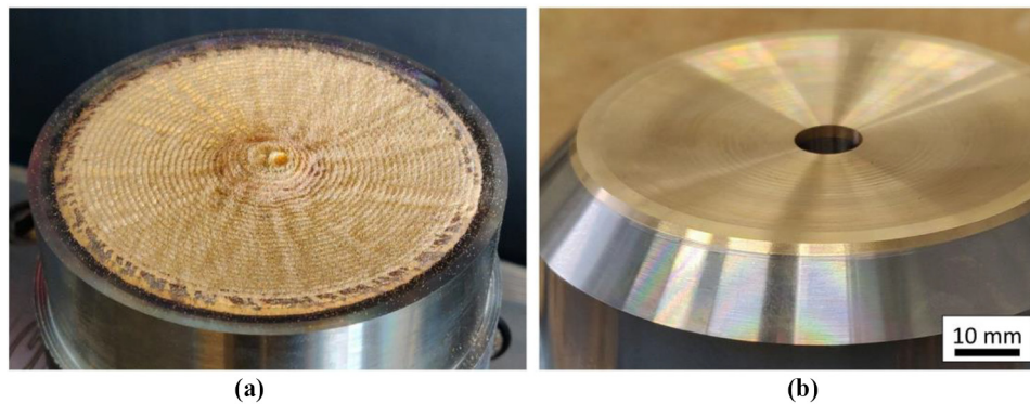
Figure 15 Hemispherical plain bearing obtained with the deposition of CuSn11 on a C45 substrate
