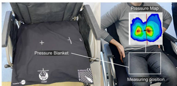
Figure 8 Pressure blanket and measurement process
