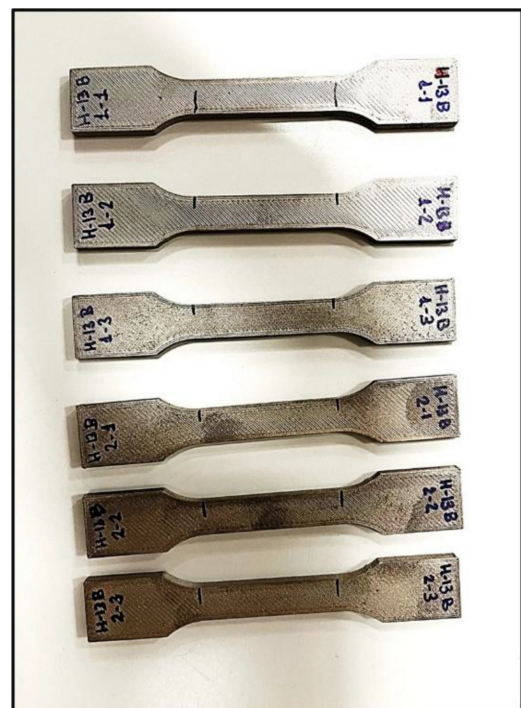
Figure 1 Tensile strength specimens prepared before testing
