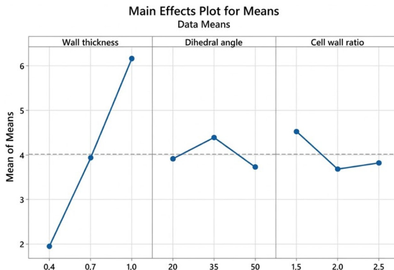
Figure 8 Effect of geometrical parameters (wall thickness, dihedral angle and cell wall ratio) on energy dissipation by ANOVA analysis
