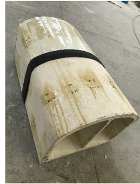
Double-line box arch tunnel
