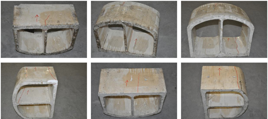
Cracked segment of lining structure (10# ~ 12#)
