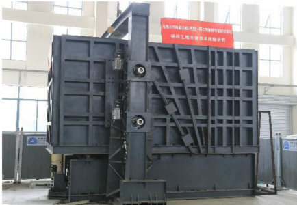
Test system to simulate loading and fault rupture (a)
