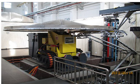
Figure 8. High-speed pantograph-catenary relationship test bench
