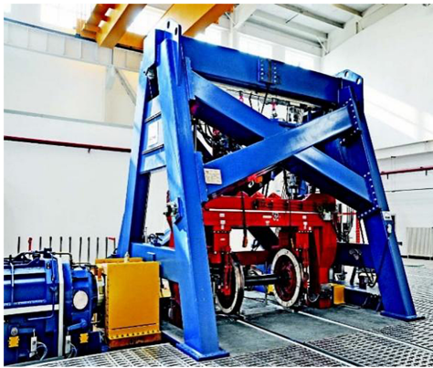
Figure 7. High-speed wheel-rail relationship test bed
