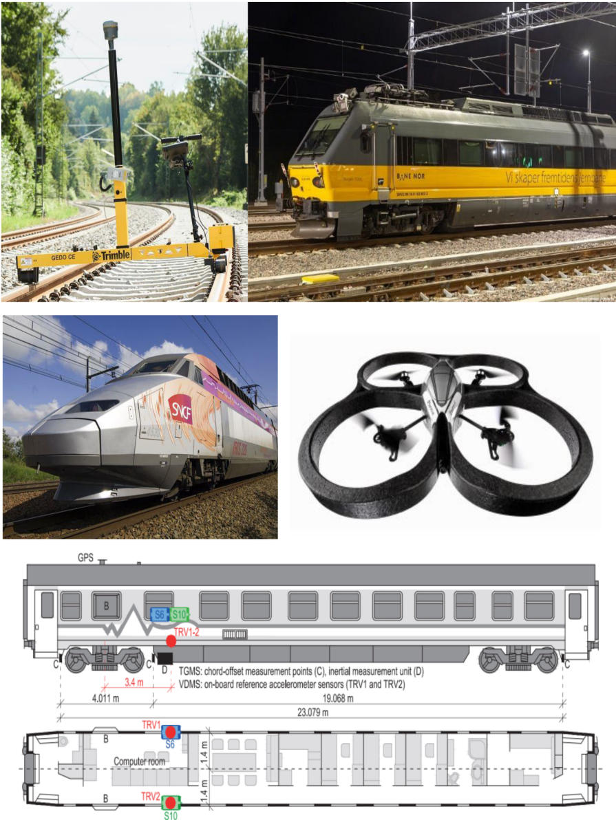
Figure 3. Classic track geometry measurement equipment (a) German GEDO CE, (b) Norwegian Roger 1,000, (c) France Iris 320, (d) Parrot AR.Drone, (e) Smartphone. Source: Figure courtesy of Trimble (2018), Gåsemyr (2018), UIC (2012), Páli et al. (2014), Vinkó et al. (2023)
