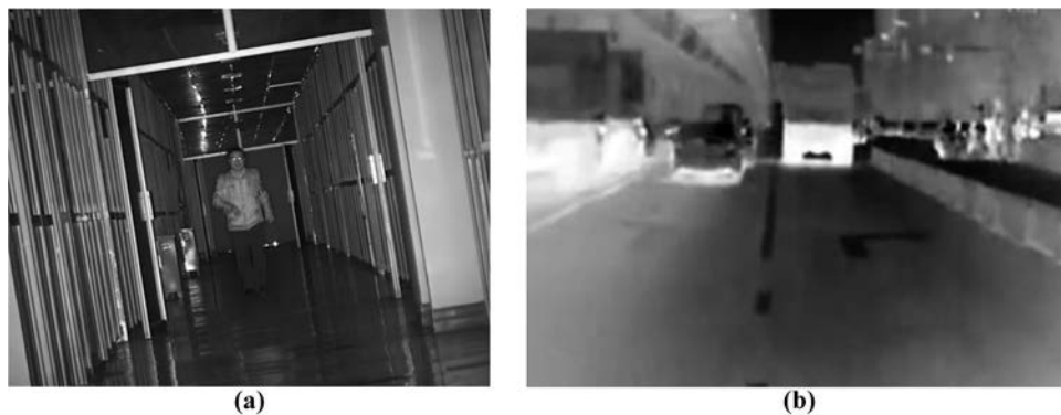
Notes: (a) Image with 940-nm near-infrared illumination at night; (b) image with long-wavelength infrared inactive at night
