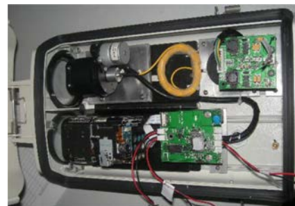
Figure 7 The composition of the IR-EDOF sensor
