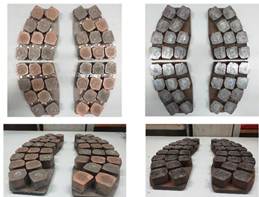
Figure 3 Examples of sintered brake pads tested at Italcertifer test rig
